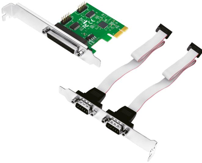
LogiLink PCI Express Card extends your PC by two serial and one parallel ports connect RS232 as well as DSUB25 compatible devices. The internal and external connections are standardized and work in any PC.
