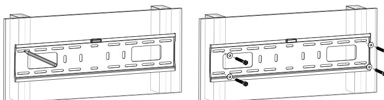
Install the wall plate to the wall
